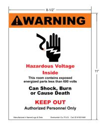
The decal shall be three colors, all colors shall be UV resistant, on 3M 7300 sheeting. The signal word panel shall have black letters on a transparent safety orange background with a transparent safety orange exclamation mark. Text copy "HAZARDOUS VOLTAGE INSIDE" and "KEEP OUT" shall be transparent safety red. All remaining text copy and symbols shall be in black.
